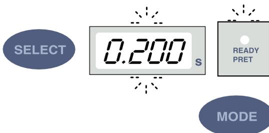
Press and **hold down** the SELECT key (about 4 seconds) until you have heard a signal tone to enter the programming mode. The time display and the ready light will start to flash.
