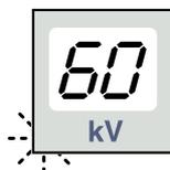
Press the SELECT key **briefly**, the kV display will start to flash and the exposure time value is stored in the memory.
