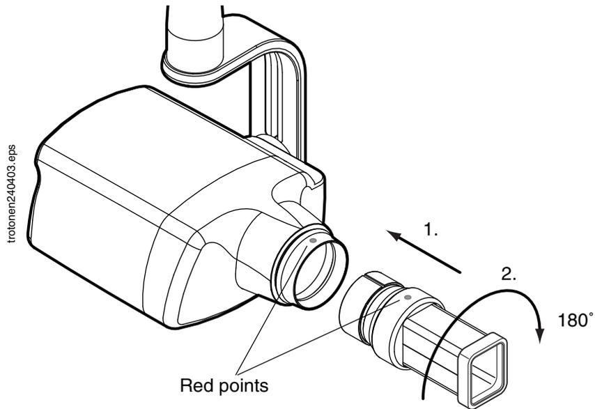
The rectangular cone can be removed when the red dots on the short cone and on the rectangular cone are in line.
