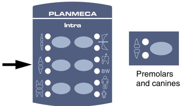
Select the premolar and canine exposure region with the preprogrammed setting keys. Press the premolar and canine key once to select the projection of the maxilla, and press the key twice to select the projection of the mandible. The indicator light of the selected projection will come on.
