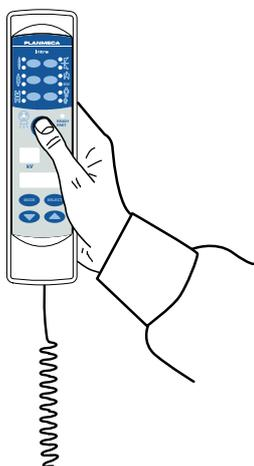
Press and hold the exposure key on the control panel for the duration of the exposure.
