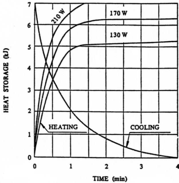
20.3.19 X-ray tube assembly heating/cooling curve
