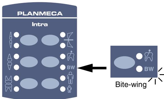
Select the bite-wing exposure region with the preprogrammed setting keys. Press the bite-wing key once to select the projection of the endo, and press the key twice to select the projection of the bite-wing. The indicator light of the selected projection will come on.
