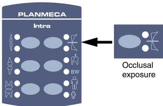
Select the occlusal exposure region with the preprogrammed setting keys. Press the occlusal exposure key once to select the projection of the maxilla, and press the key twice to select the projection of the mandible. The indicator light of the selected projection will come on.
