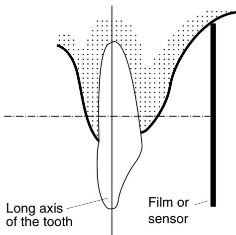
The film or sensor is placed to a film holder which is used to align the film parallel to the long axis of the tooth.
