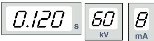
After the self-test is completed the default exposure values will appear on the displays.
