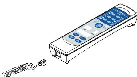
One end of the control panel cable is connected to the terminal at the underside of the generator box, and the other end to the control panel.
