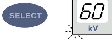
Press the SELECT key **briefly**, the kV display will start to flash and the exposure time value is stored in the memory.
