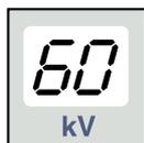
The selected kV value is shown on the kV display. There are eight different values that can be selected: 50, 52, 55, 57, 60, 63, 66 and 70 kV.
