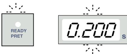
The ready light will start to flash. The time display will start to flash and the default exposure values will appear on the displays.
