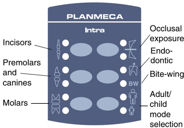
Select the exposure region with the preprogrammed setting keys. Press the desired key once to select the projection of the maxilla, and press the key twice to select the projection of the mandible. The indicator light of the selected projection will come on.
