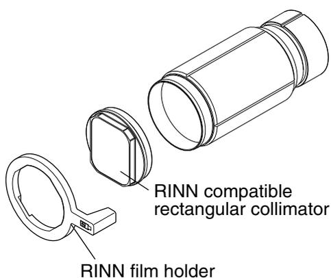
Attach the RINN compatible rectangular collimator to the long cone. The film holder can be attached to the collimator.
