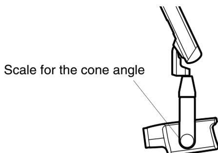
The angle of the cone is indicated on the scale located on the vertical joint of the tube head.
