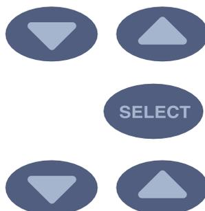
The preprogrammed time, kV and mA values can be temporarily changed with the parameter adjustment keys. This will not affect the preprogrammed values.
