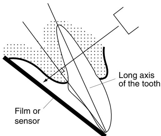
The patient holds the film or sensor in place with his finger. The X-ray beam is directed perpendicularly towards an imaginary line which bisects the angle between the film plane and the long axis of the tooth.
