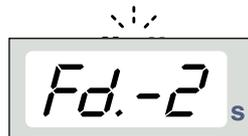
When the SELECT key is pressed a third time **briefly**, the current density value starts to flash on the time display and the mA value is stored in the memory.
