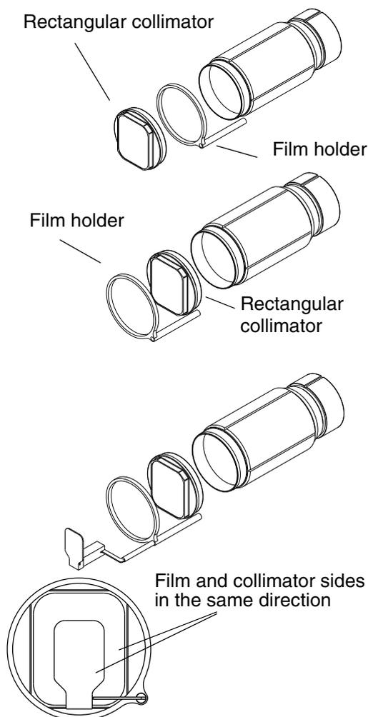
The rectangular collimator can be attached to the long cone either before the film holder or after it. When the collimator is attached before the film holder, the film holder rotates when the collimator is rotated.
