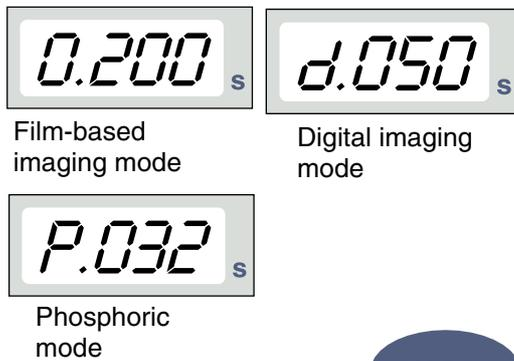
Check that you are in the desired mode: in the film-based imaging mode, in the digital imaging mode or in the phosphoric mode.
