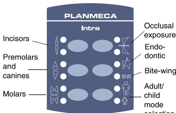
The unit is preprogrammed with exposure parameters - time, kV and mA values - which can be selected by pressing these keys. There are ten sets of parameters for both the child mode and the adult mode: one for each exposure region and one for default exposure values, which are in use when an exposure region is **not** selected.
