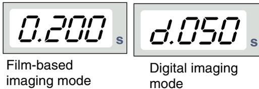
Check that you are in the desired mode: in the film-based imaging mode, in the digital imaging mode or in the phosphoric mode.
