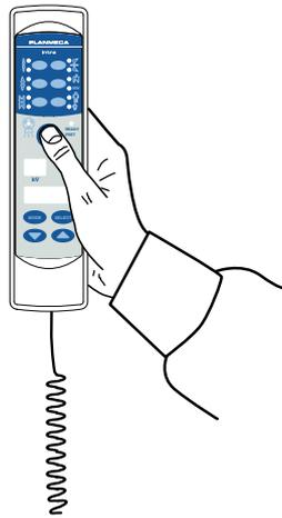
Press and hold down the exposure key on the control panel for the duration of the exposure.
