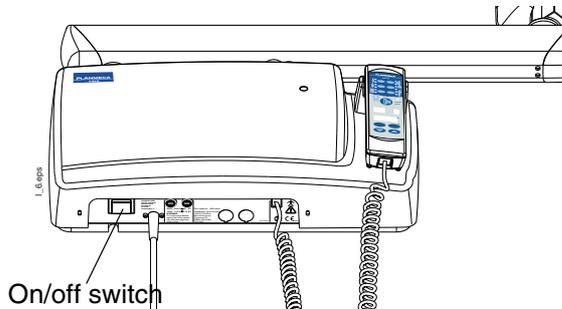
The on/off switch is located under the generator box. When the unit is switched on it will carry out an automatic self-test during which the Display CPU software version is shown on the kV display, and the Tube head CPU software version on the time display.
